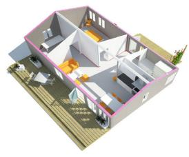
For the house's exterior and interior walls, sandwich element panels consisting of two solid fiber cement boards insulated with expanded polystyrene (EPS) were chosen. The pre-fabricated roof panels consist of polyisocyanurate (PIR) insulated reflective steel with gutters that collect rain water for reuse.
